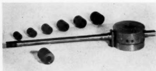
FIG. 1. Condenser unit of ionometer with 1 cubic centimeter graphite chamber of various wall thicknesses.
